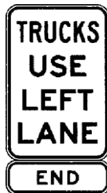
End trucks use left lane sign
